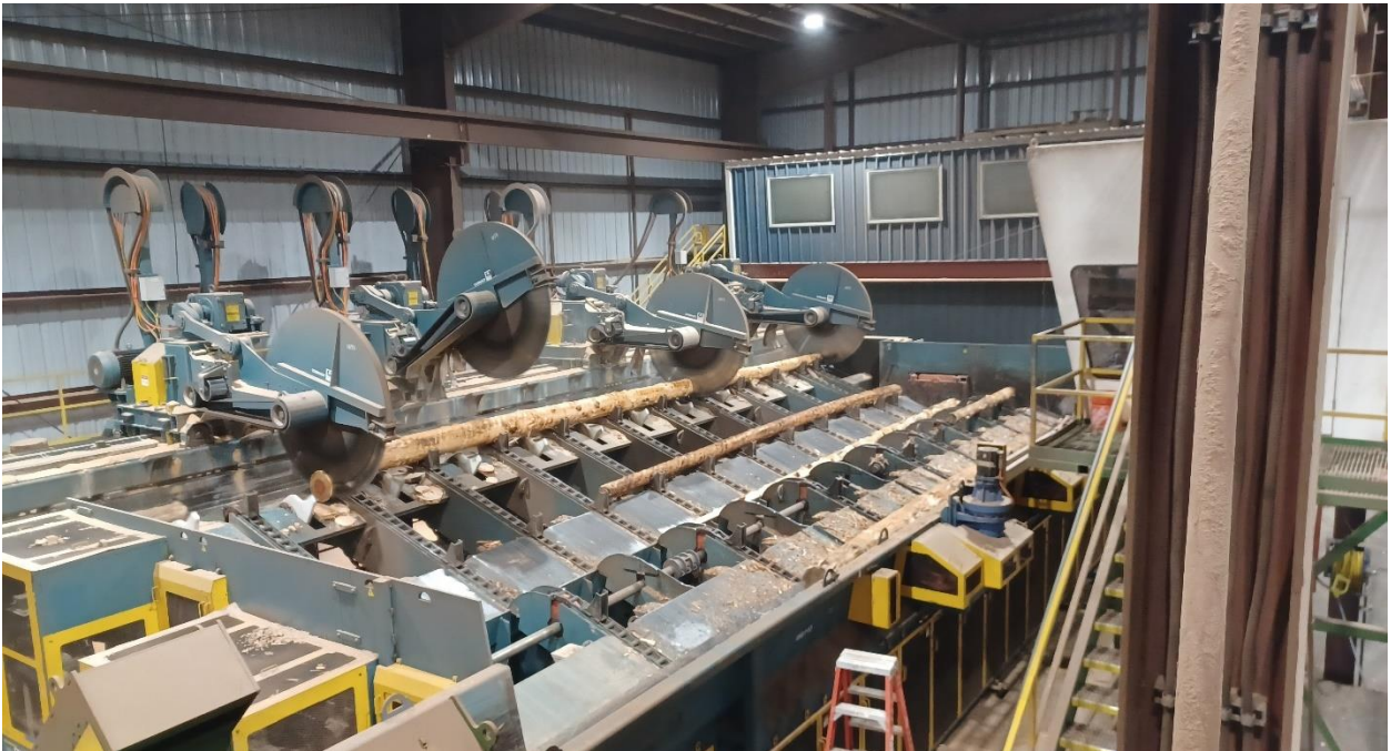
One of the two mills on the Sierra Pacific site is this new fully automated cut-to-length system used for making dimensional lumber.
