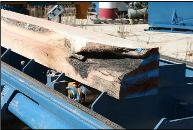
Marschall instructed the sawyer to ignore the fire damage and cut for the highest grade possible.
