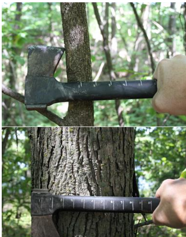
Figure 1: (top) Measuring small diameter trees from the lower tip of the hatchet blade using a ruler engraved/painted on the handle. (bottom) Measuring larger diameter trees using an engraved/ painted Biltmore-stick-style scale on the opposite side of the hatchet handle.
