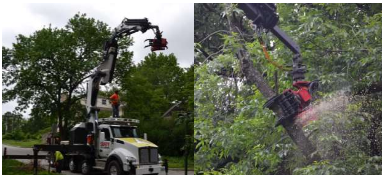
Left: Safety Tree Service staff demonstrate the agility of the scorpion crane, which is a huge benefit for removing trees in tight spaces. Right: The cutting head features a double-grapple head and chainsaw cutting bar.
